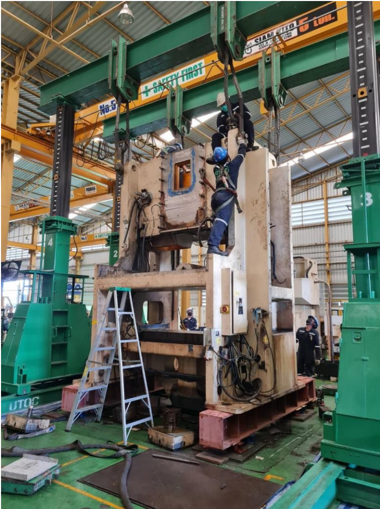
600 Ton Patec Press (Bolster 2100 x 100 mm) Machine Weight : 68 ton Orii 3-in-1 Leveller Feeder (max thickness : 9.0 mm. Width : 600)
